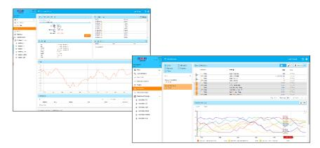
An Alarms page will provide details of any active alarms and give the ability to search for previous alarms. You will be able to acknowledge the alarms and see the duration of the alarms.
