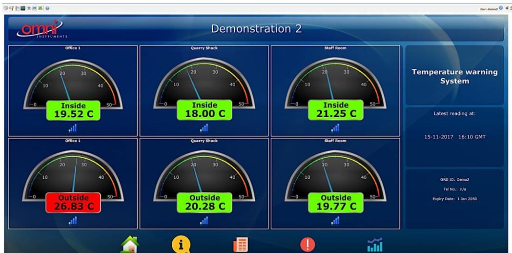
Data from the data logger can be viewed on the M2M web interface in chart, table and graphical format. The data can also be downloaded as a CSV file. The web interface provides a data panel where customers can view a customised web interface showing data from all their remote locations. The channel scaling, reports, alarm levels, and alarm recipients are set from our web control page removing the need to dial up units or visit sites for reprogramming.
